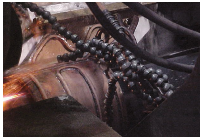
Figure 2: The tube passing through the high-frequency induction coil
