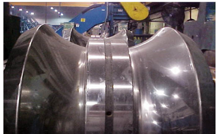
Figure 1: A typical fin pass roll
